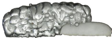
Figure 1 Aluminum component with monolithic salt support structure. Height of the component: approx. 5 mm.
