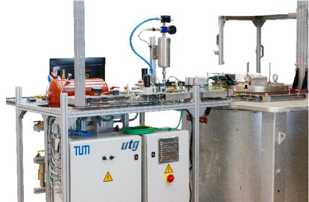
Figure 1: Research low-pressure casting machine for casting squirrel-cage rotors, minimum casting time < 1 s at more than 50 mbar/s
