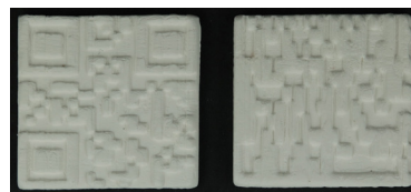
3D printed barcode inserts ©Fraunhofer IGCV
